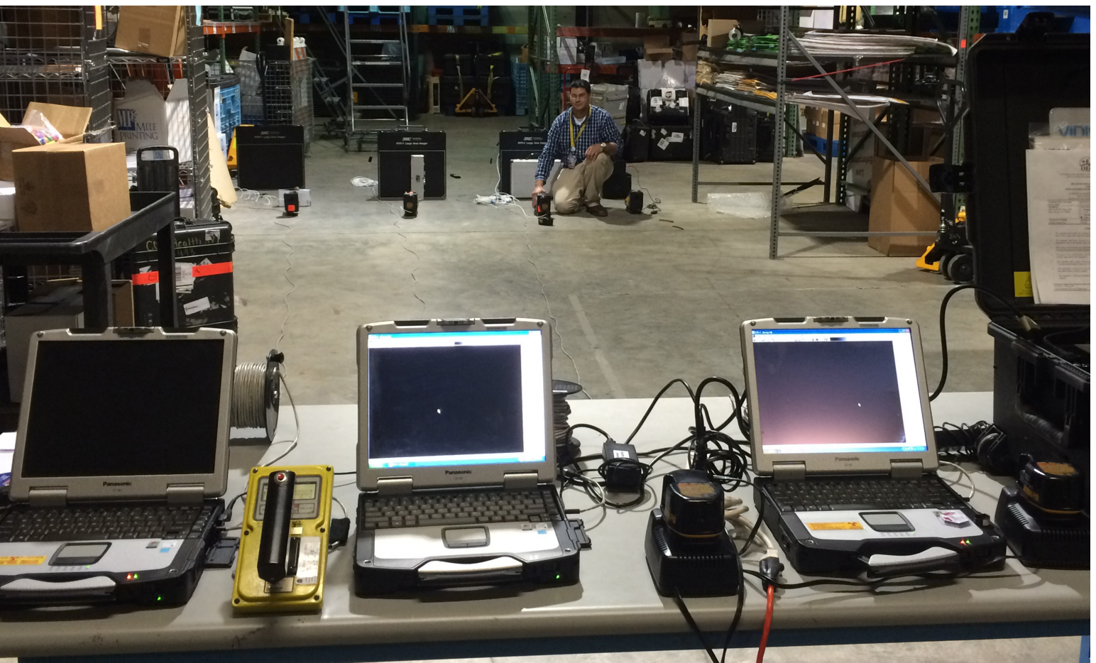
RSO radiation specialist Amin M. Hamideh conducts inspections on portable digital X-ray systems, used for detecting explosives, weapons, narcotics, and other contraband at the LSU National Center for Biomedical Research and Training.
